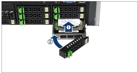
Figure 26: Installing the 2.5-inch HDD module
